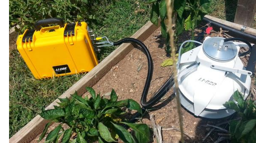
Figure 3. Automated soil flux system, Licor 8100a
