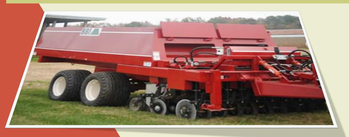
The USDA-ARS Subsurfer evolved from prototypes that successfully placed dry poultry litter below the soil surface with limited soil disturbance. The technology uses a system of augers to convey and grind dry litter (<25% moisture), and a combination of no-till planting components to incorporate the litter.
