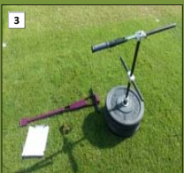
Photos 3-4, Canaway device to measure rotational resistance; Photos 5-6, TAFT device to measure horizontal and vertical force.
