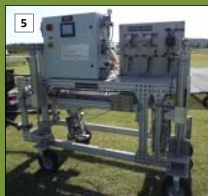
Photos 3-4, Canaway device to measure rotational resistance; Photos 5-6, TAFT device to measure horizontal and vertical force.
