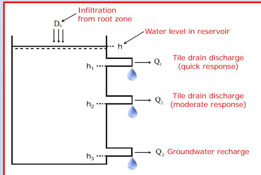
Fig. 2. Linear reservoir with three outlets. Infiltration out of the root zone was calculated by a simple root zone water balance model, EVACROP (Olesen and Heidmann, 1990) using soil type, land use, and climatic data as inputs.
