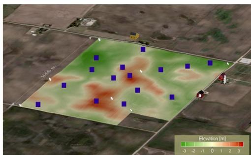
Our field site just outside of Ames, IA has been instrumented with soil moisture sensors, precipitation gauges, a flux tower, wells and a COSMOS cosmic-ray detector. It is maintained in a traditional corn-soybean rotation with chisel plow tillage.
