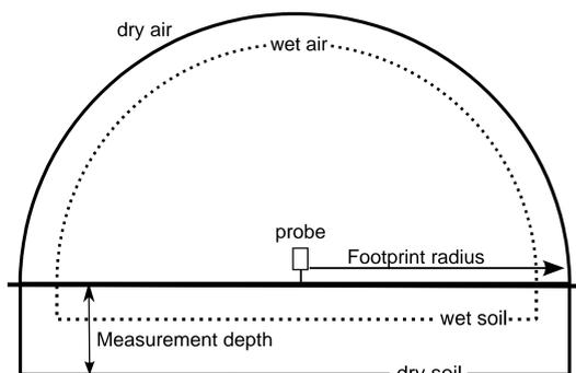
A diagram of the sensitivity of the cosmic-ray neutron detector. Adapted from Ochsner et al. (2013).
