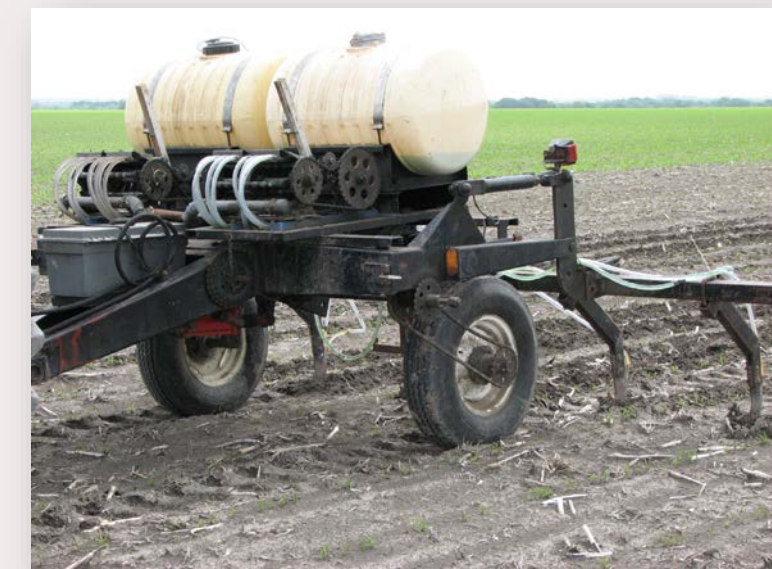
Plate 1. Giddings hydraulic soil probe and ground-driven, liquid fertilizer applicator used in all studies.
