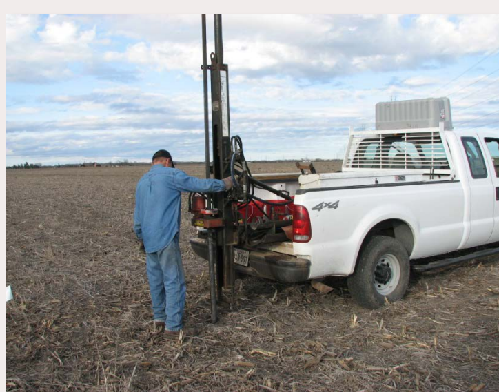
Plate 1. Giddings hydraulic soil probe and ground-driven, liquid fertilizer applicator used in all studies.
