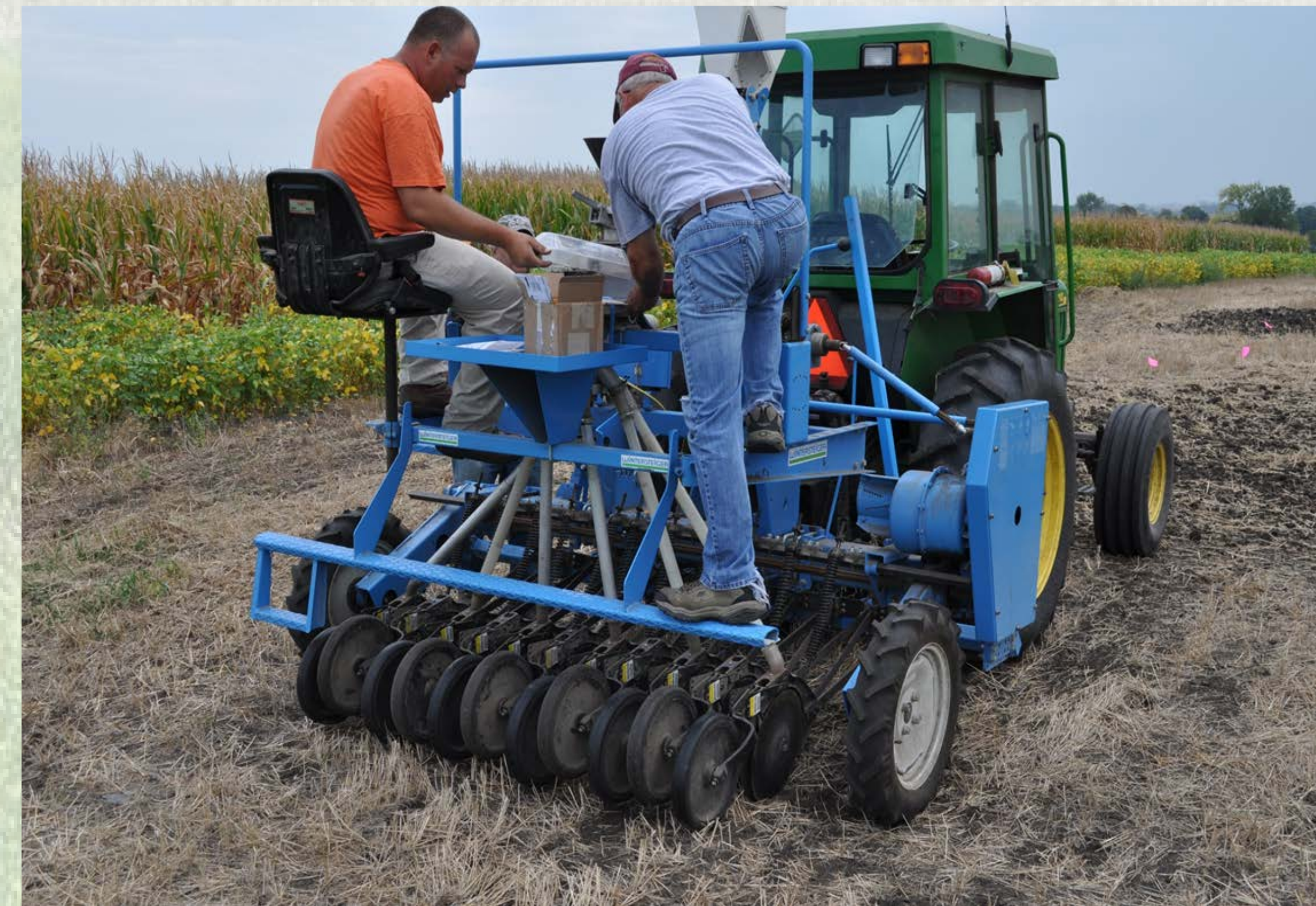
Test plots were planted with a Wintersteiger plot drill with double-disk openers
