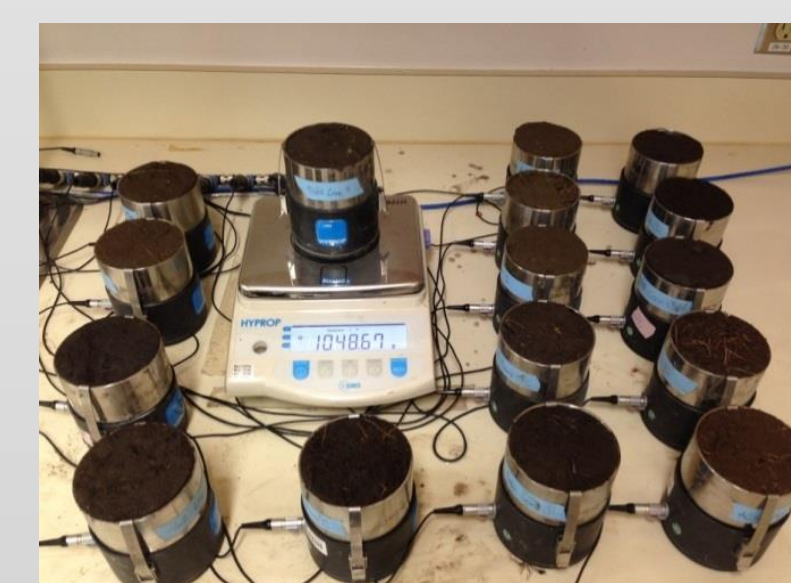
Figure 4. Hyprop campaign measuring the water loss and water tension due to evaporation.
