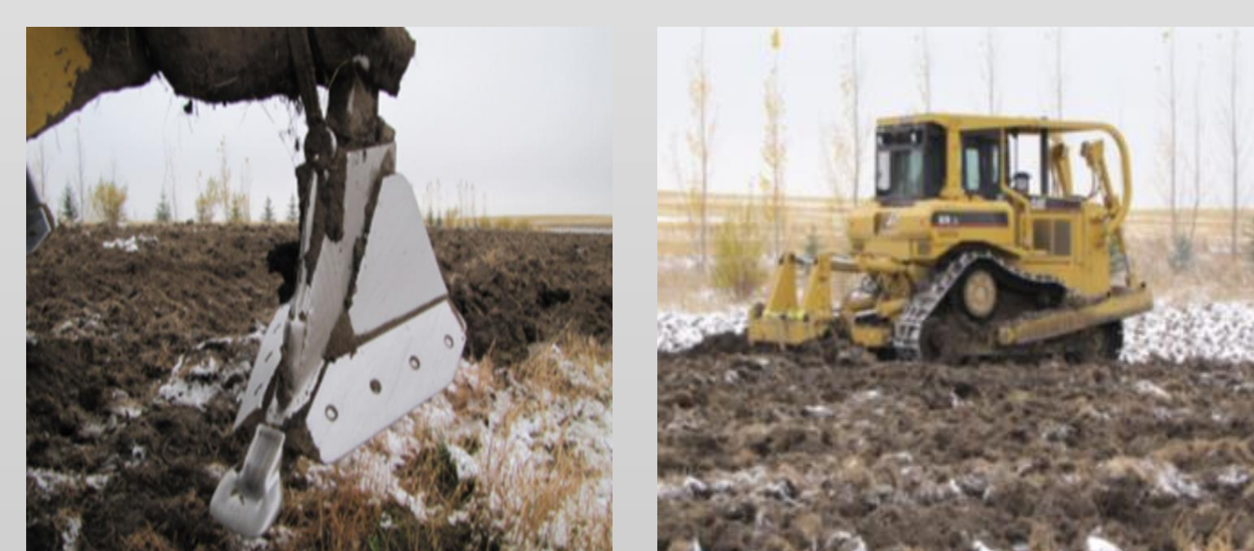
Figure 1. A McNabb Winged Subsoiler D7R XR Caterpillar used for sub-soil ripping of compacted soils in the fall of 2010 at Genesee Prairie Mine, AB. Sub-soil ripping was completed to a 60 cm depth.
