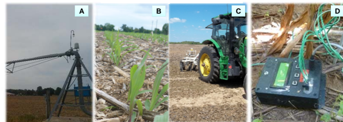
Figure 4. Field study (A and B), Veris-electrical conductivity measurement (C) and Arduino instrument used to measure soil water potential (D).
