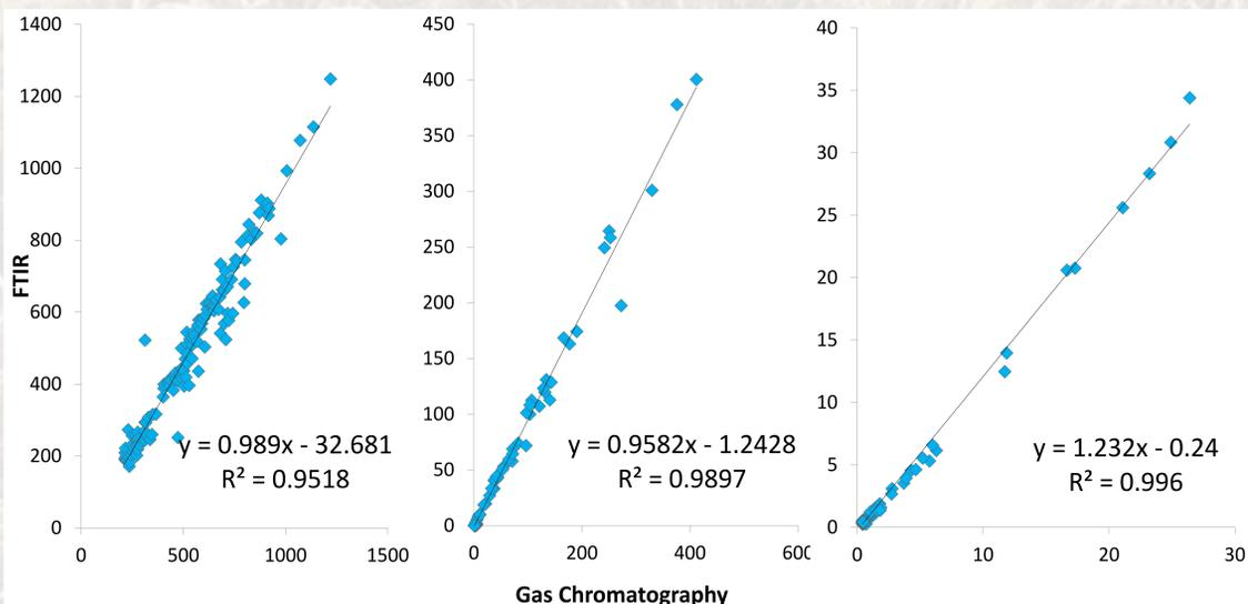
**Figure 2.** CO<sub>2</sub>, CH<sub>4</sub>, and N<sub>2</sub>O concentration comparisons from 133 paired GHG measurements from FTIR (y-axis) and GC (x-axis).
