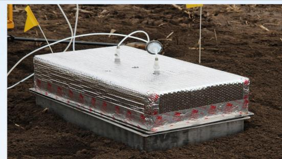
**Figure 1.** Greenhouse gas chambers, constructed of stainless steel, were used consistently at all sites. Chamber anchors were deployed at least 24 hours in advance of measurements. Chamber lids for this experiment were outfitted with a rubber gas sampling septa for syringe based sampling and two Teflon tubing fittings for FTIR tubing to attach to the chamber.
