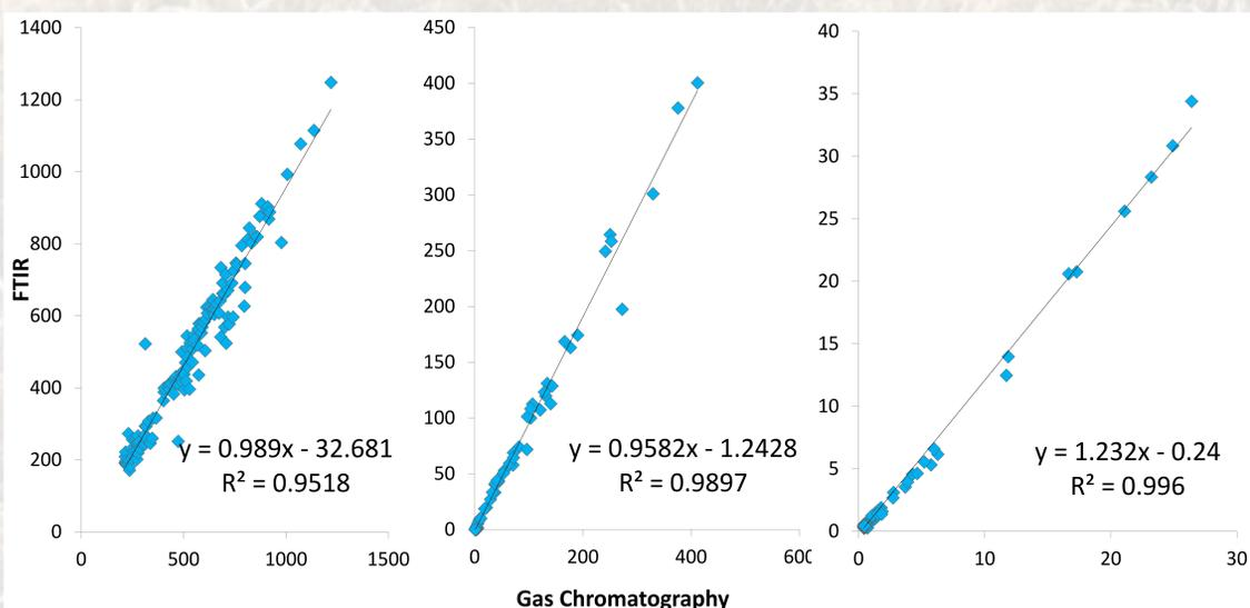
**Figure 2.** CO<sub>2</sub>, CH<sub>4</sub>, and N<sub>2</sub>O concentration comparisons from 133 paired GHG measurements from FTIR (y-axis) and GC (x-axis).
