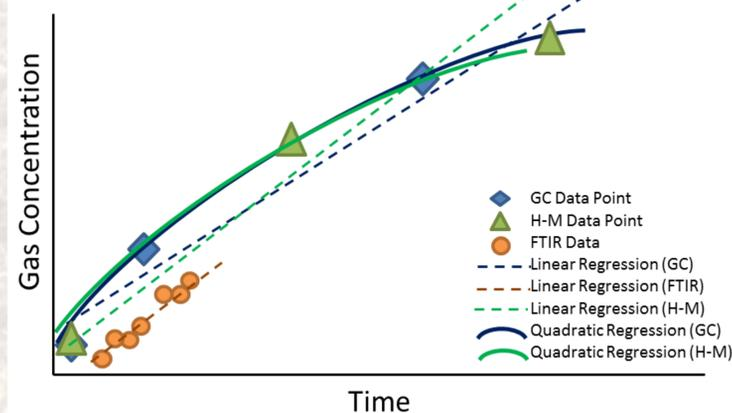
**Figure 3.** This schematic shows how variable flux regressions can be, from FTIR and GC collection (H-M is considered a subset of GC points, with only three data points used to determine flux) and between regression models from linear to quadratic and H-M calculations.
