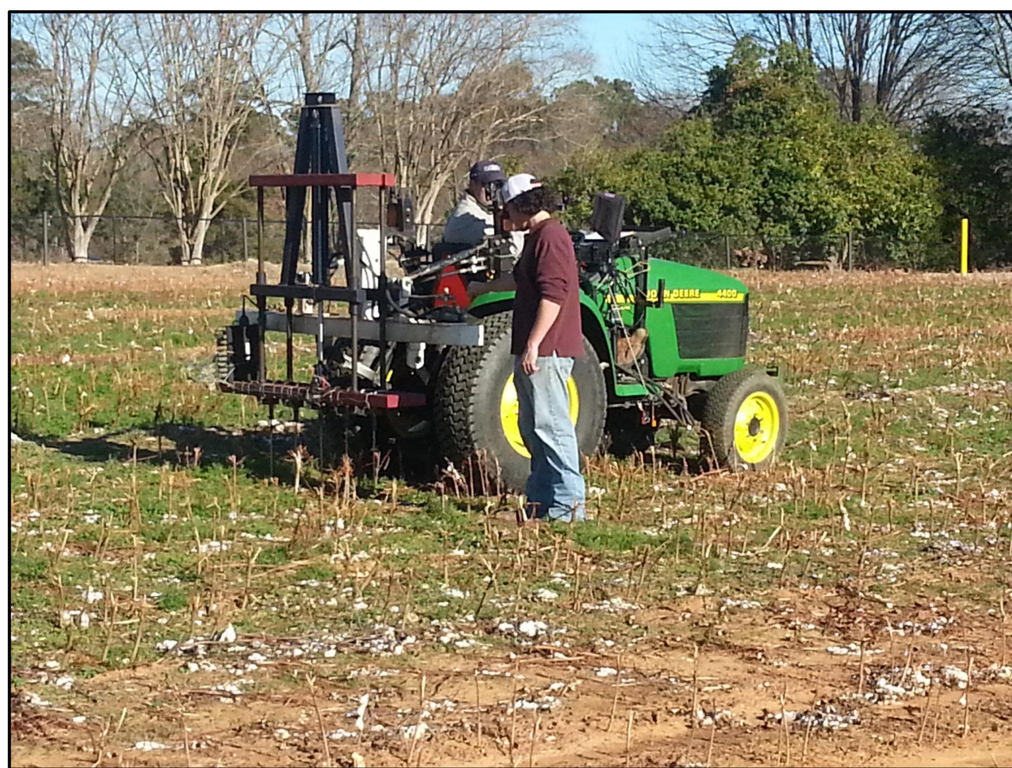
Fig. 1. Soil strength measurements collected with a multi-probe soil penetrometer (Raper et al., 1999) from the Old Rotation on 12 December 2014 in Auburn, AL
