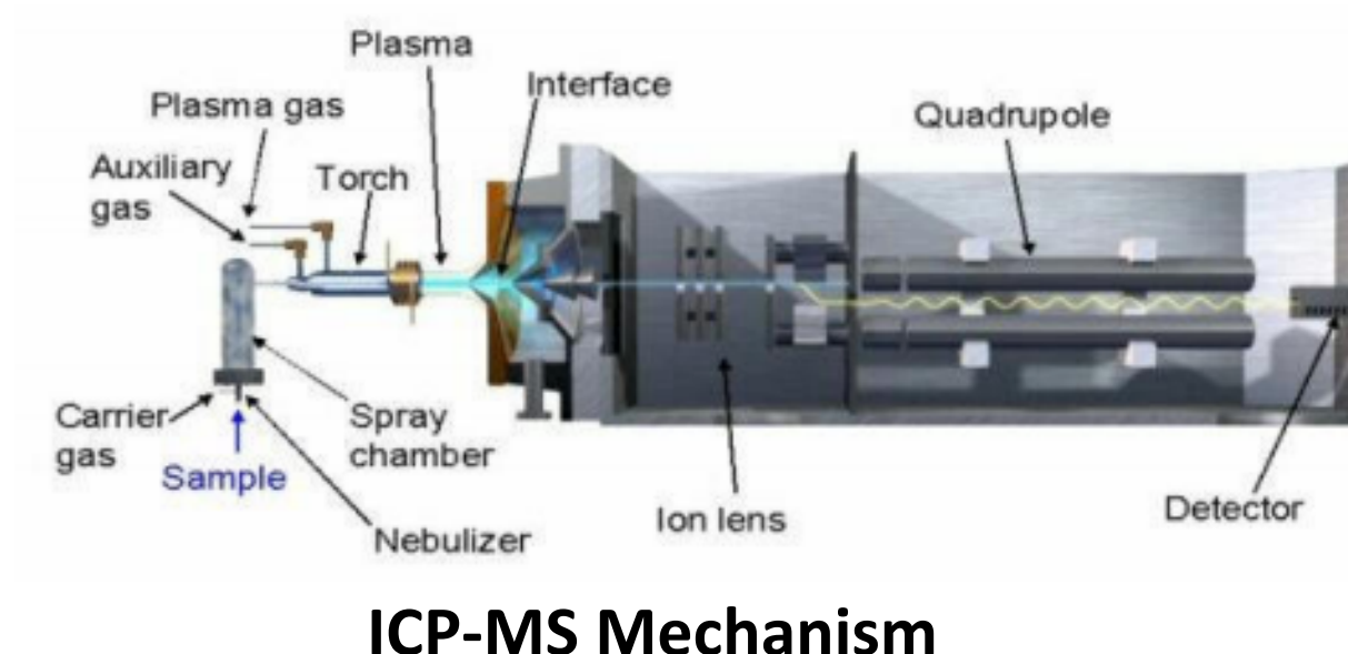
ICP-MS Mechanism
