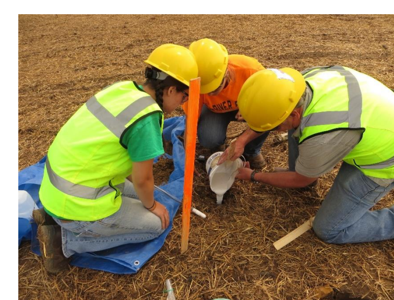
Figure 4: Installation of lysimeter.
