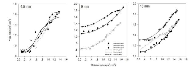
Fig. 5 SSCs (Eq. [2]) with different samples thicknesses
