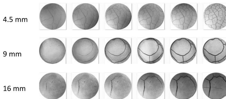
Fig. 2 The cracking process of soil samples with different thicknesses
