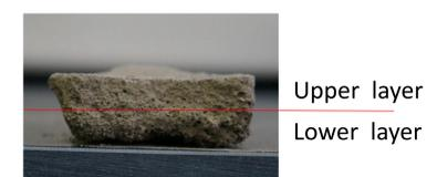
Fig. 7 A picture of the 16-mm-thick soil sample showing the nonuniform distribution of water.
