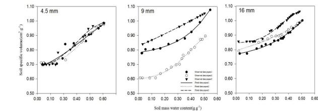
Fig. 6 SSCs (Eq. [3]) with different samples thicknesses
