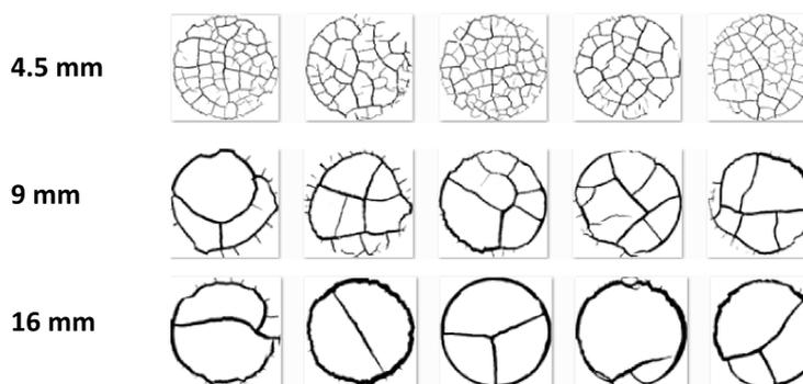
Fig. 3 Crack morphologies with different sample thicknesses
