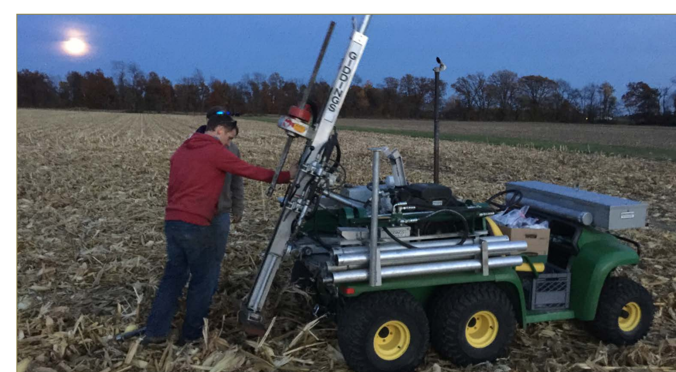
Fig. 2 Soil sampling unit used to take deep cores.
