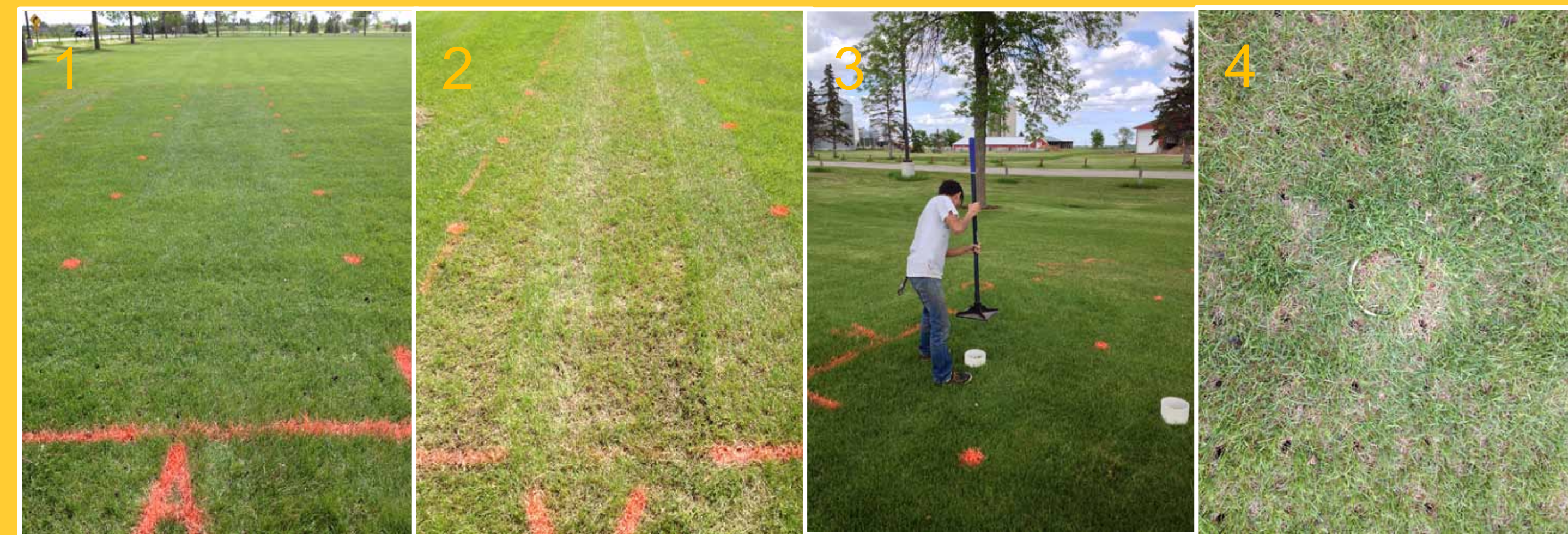
Photo 1: For the aeration treatment, plots were aerified each September and May. Photo 2: For the verticutting treatment, plots were also verticutted each September and May. Photo 3: At the beginning of the study, anchors were tamped into the soil surface to create a good seal with the greenhouse gas chambers on sampling days. Photo 4: Anchor tamped into the soil surface of an aeration plot.
