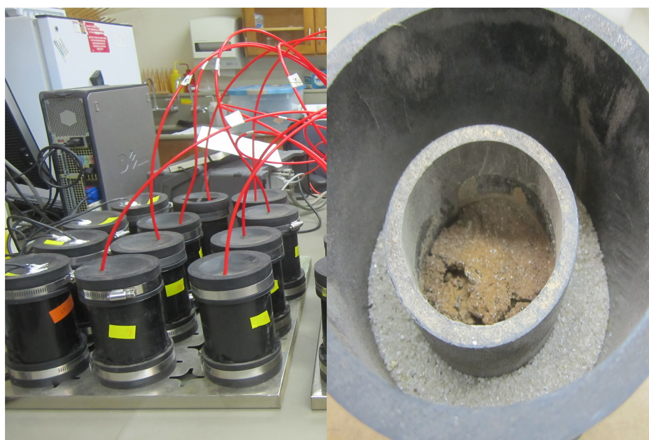
Figure 2: 4cm diameter PVC cylinder nested within the 7.75cm cylinder with sand filling the medium to allow for air flow during sampling.
