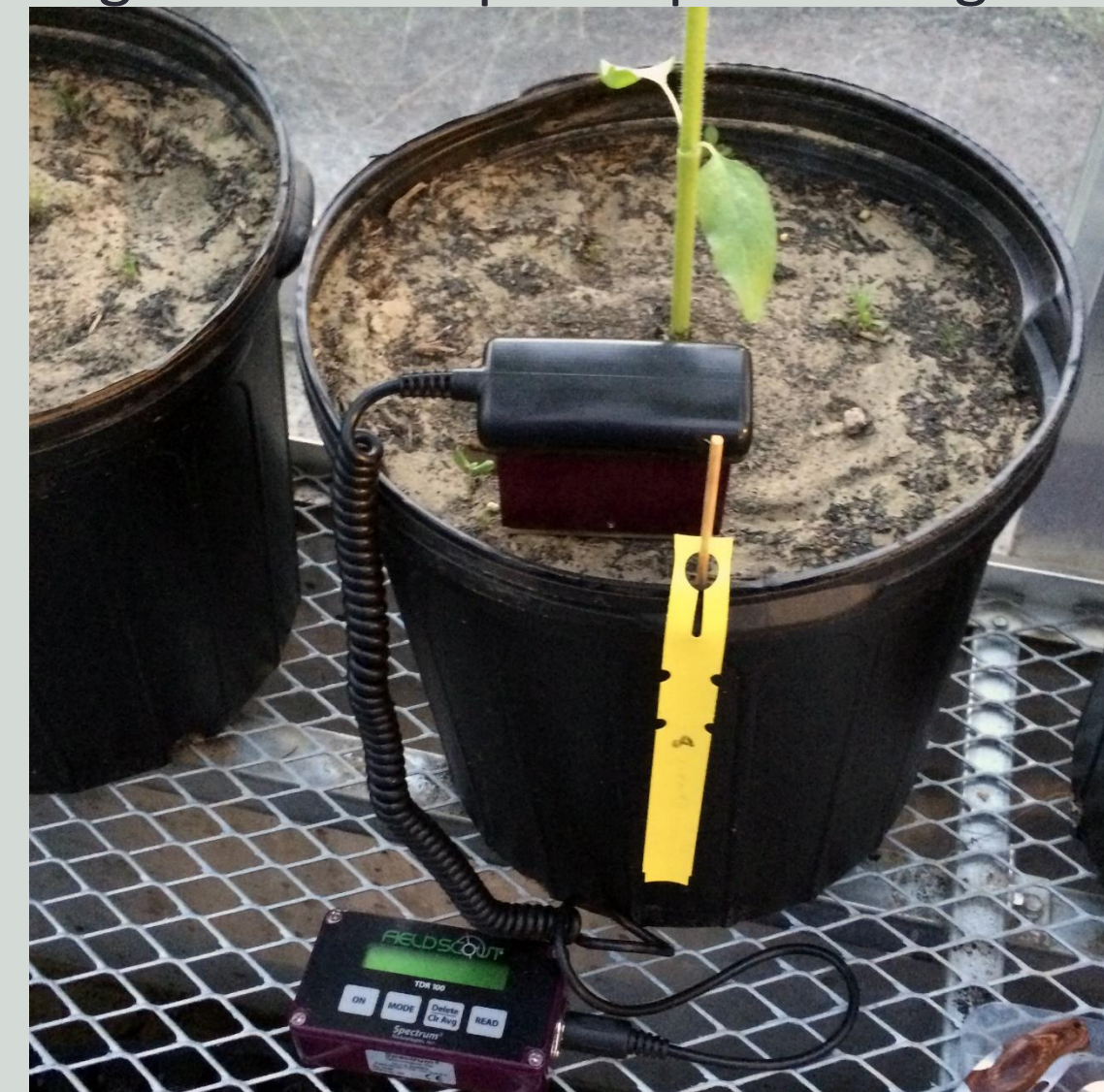
Figure 9: Soil moisture reading
