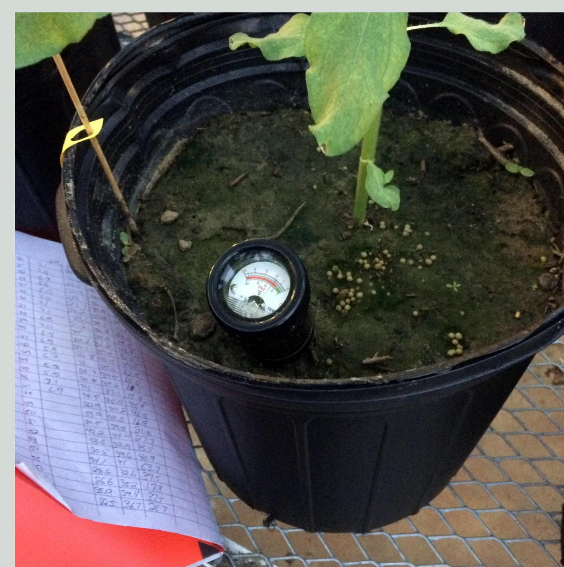
Figure 7: Field probe pH reading
