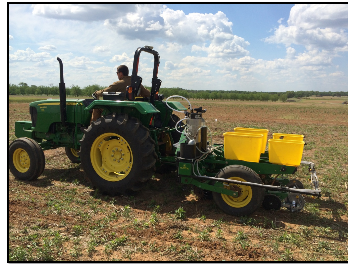
Figure 1. John Deere Planter with liquid starter setup.
