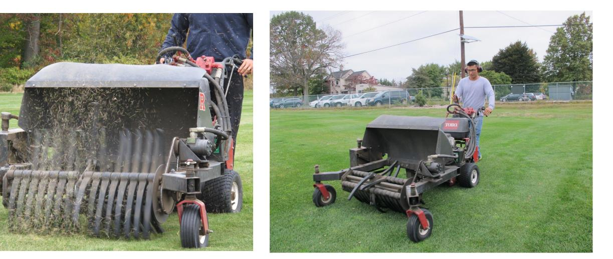
The abrasive wear applied by Rutgers Wear Simulator (RWS) causes crushing and tearing on turf plot
