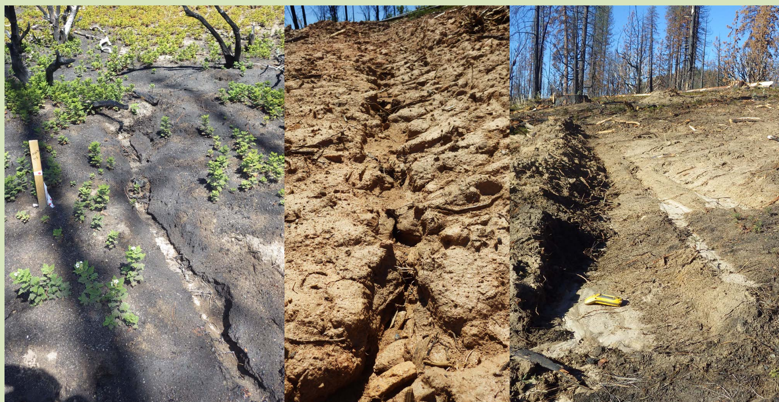
Fig. 1: Rill erosion in a burned area one year post-fire (left), in a high traffic skid trail (center), and diverted by a waterbar in a skid trail (right).
