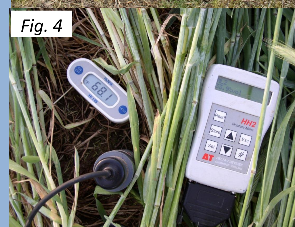
Figure 3: Soybean trial ready to be planted into early terminated (left) and standing green (right) rye at a farmer cooperator's in east-central PA. Figure 4: A digital thermometer and moisture meter were used to measure soil temperature and volumetric water content in the top 8 cm. of soil multiple times throughout the growing season.
