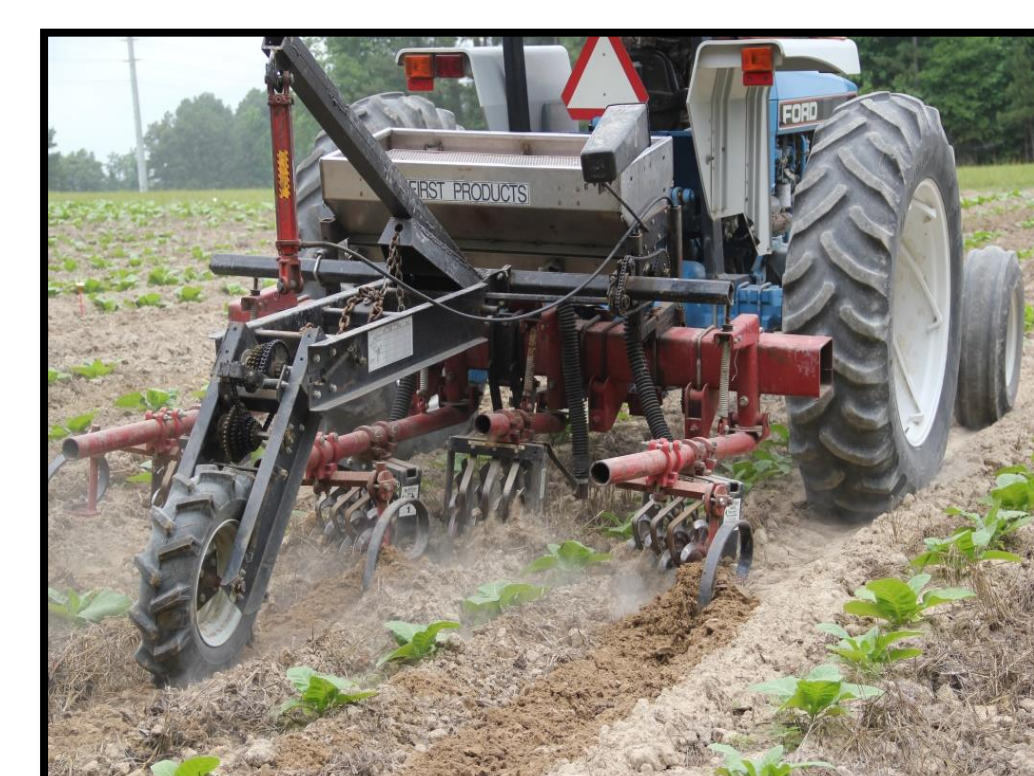
Figure 5. Rolling spider cultivator was used to apply sidedress fertilizer (17 kg ha -1 of 15-0-15) at 2 nd cultivation.
