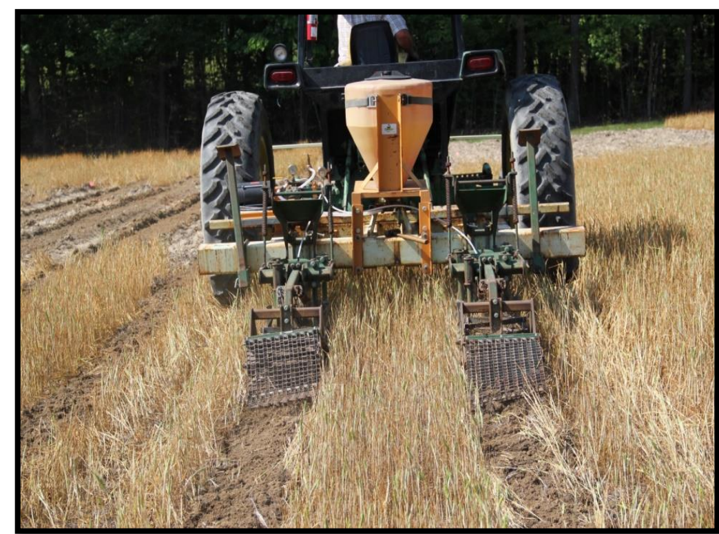
Figure 1. Strip-tillage rows were prepared with a two-row strip-till rig into a wheat cover crop.
