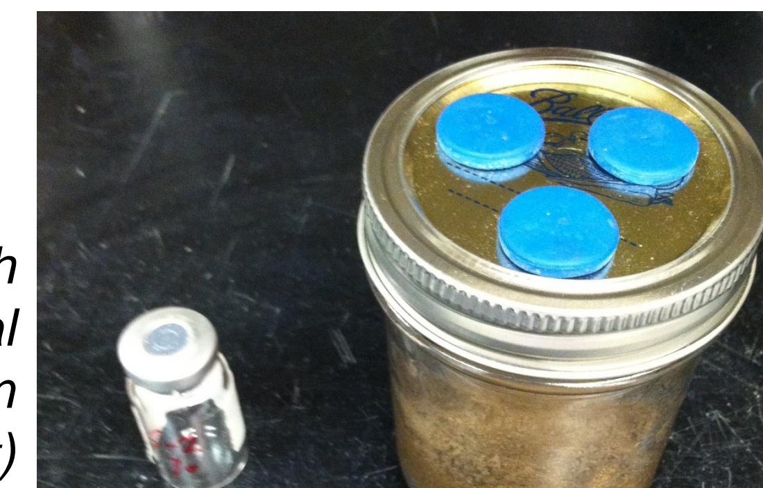
Top: Gas chromatograph Bottom: 5mL gas sample collection vial (Left) and individual soil sample incubation container with rubber septa (Right)
