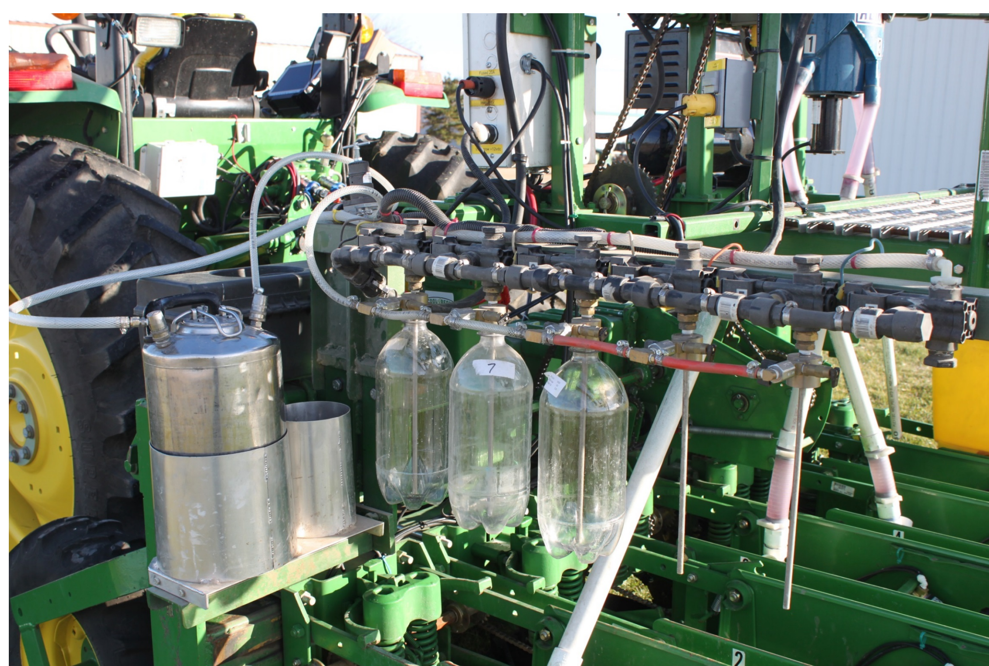
Figure 6. Liquid in-furrow application system with 3 l bottles, electric valves, and optional 11 l bulk application tank.
