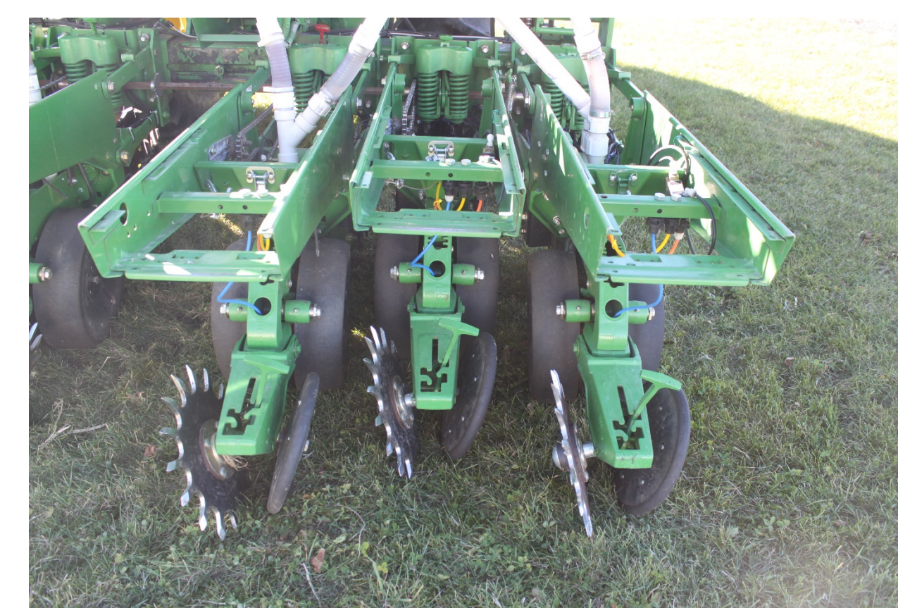
Figure 4. Row units with closing wheels in 38 cm configuration.
