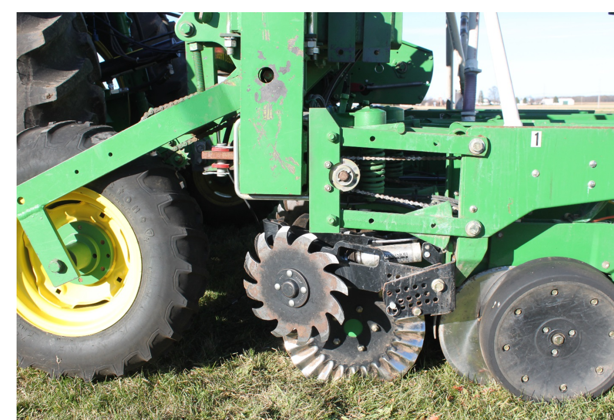
Figure 5. Drive wheel and John Deere XP row unit with no-till coulter, row cleaner, furrow opening disk blades, and depth wheel.
