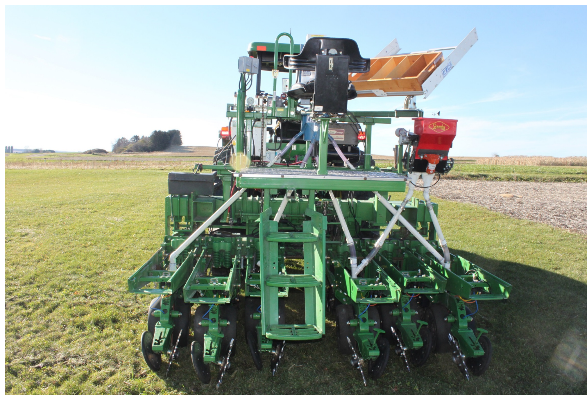
Figure 3. Rear view with operator platform, seed box, 76 cm row configuration, and dry inoculator.
