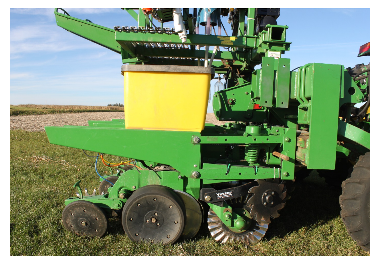
Figure 8. Bulk seed planting configuration with 55 l hopper.
