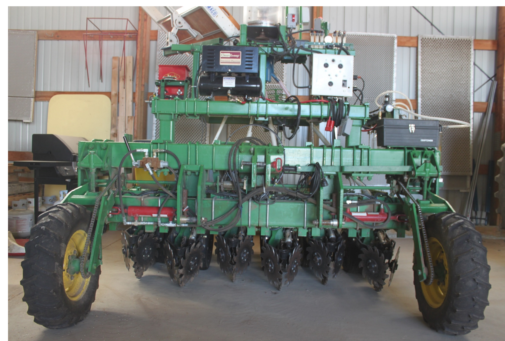
Figure 2. Front of planter showing hitch, frame, drive wheels, and row spacing adjustment mechanism.
