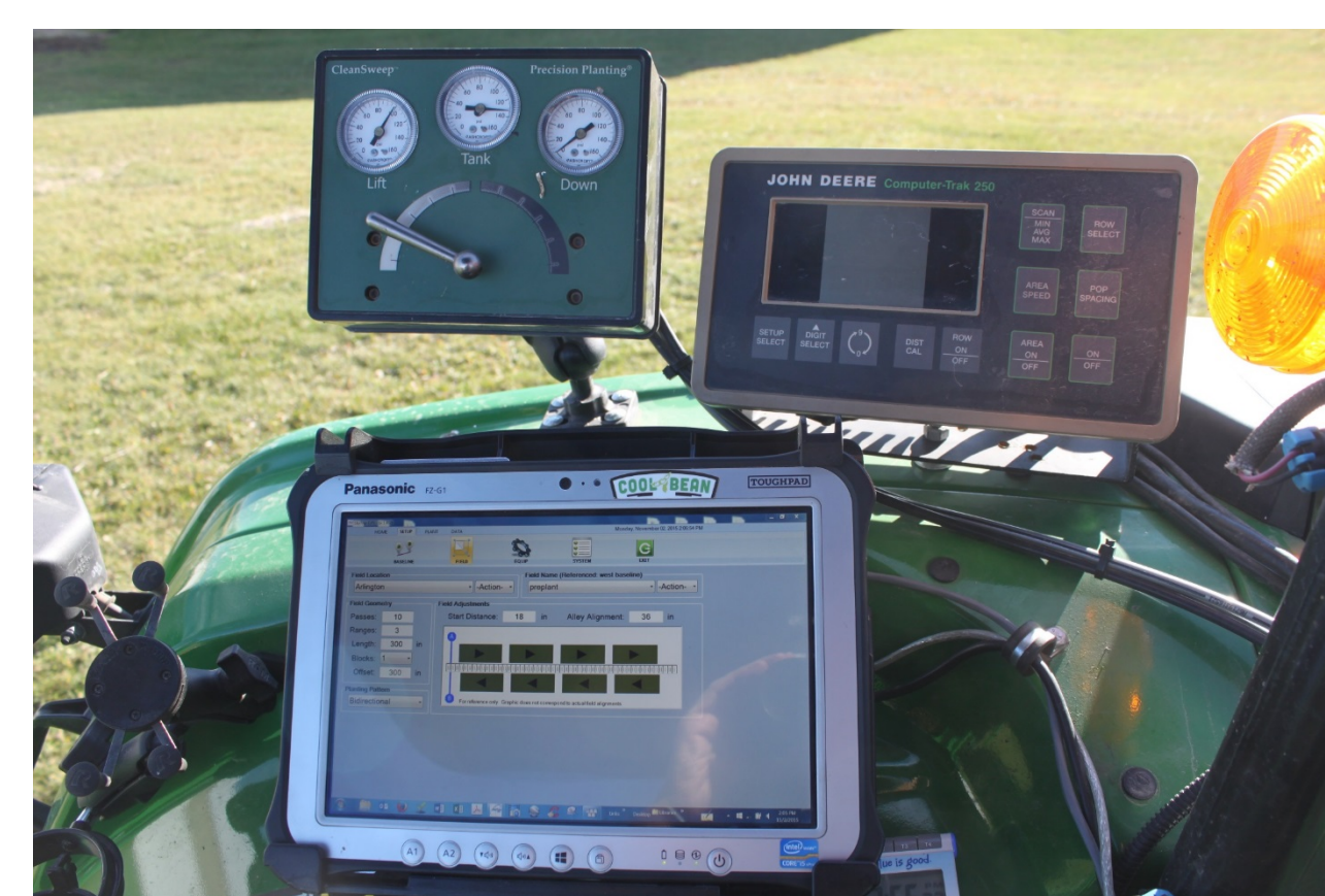
Figure 7. Clockwise from top left: row cleaner height adjustment control, Computer-Trac monitor, and tablet computer with SkyTrip plot software.
