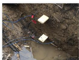
Sensors for soil volumetric water content measurement at 5 and 25 cm
