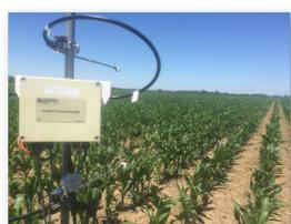
Flux gradient method for  $N_2O$  measurement
