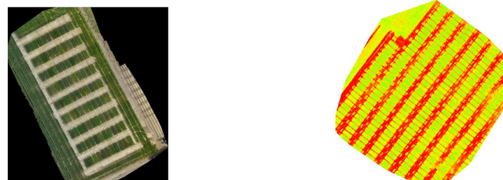
Figure 4: The orthomosaic of RGB images (left) and aerial NDVI (right). RGB altitude was at 10 m with 75% x 90% overlap. NDVI altitude was at 20 m with 75% x 75% overlap.
