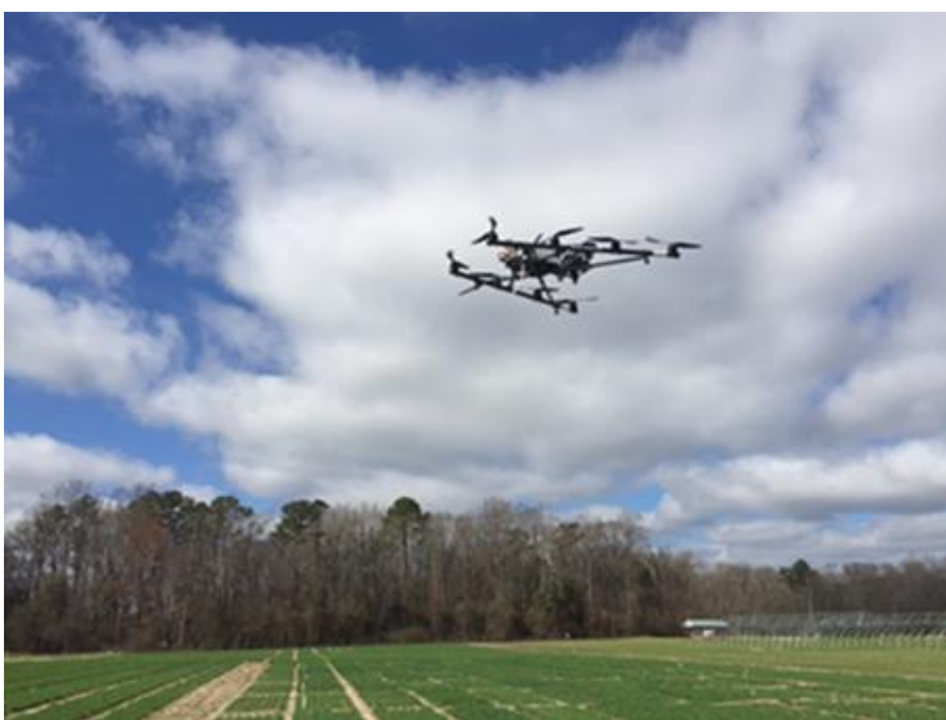
Figure 1: AscTec Falcon 8 flying and collecting data over wheat plots in Suffolk, VA.
