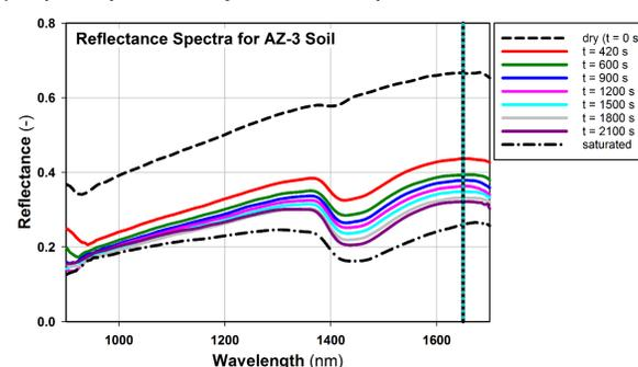
Figure 3: A series of reflectance spectra for AZ-3 soil. Measurements were conducted with the 0.5 cm deep sample container and a syringe pump discharge rate of 0.5 ml min<sup>-1</sup>.
