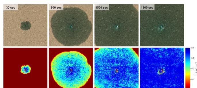
Figure 4: Surface moisture distribution maps for AZ-3 soil.
