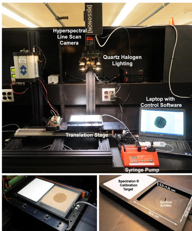
Figure 1: Experimental setup with close-up views of a sample container (during acquisition the sample moves relative to the steady camera).
