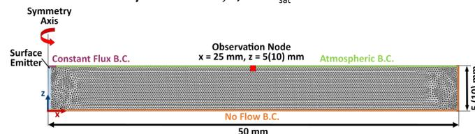
Figure 2: Simulation domain with applied boundary conditions.
