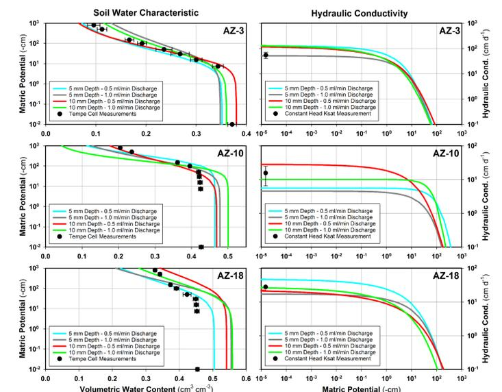
Figure 5: Comparison of inversely derived  $\theta(h)$  and  $K(h)$  functions with Tempe cell and constant head permeameter measurements.
