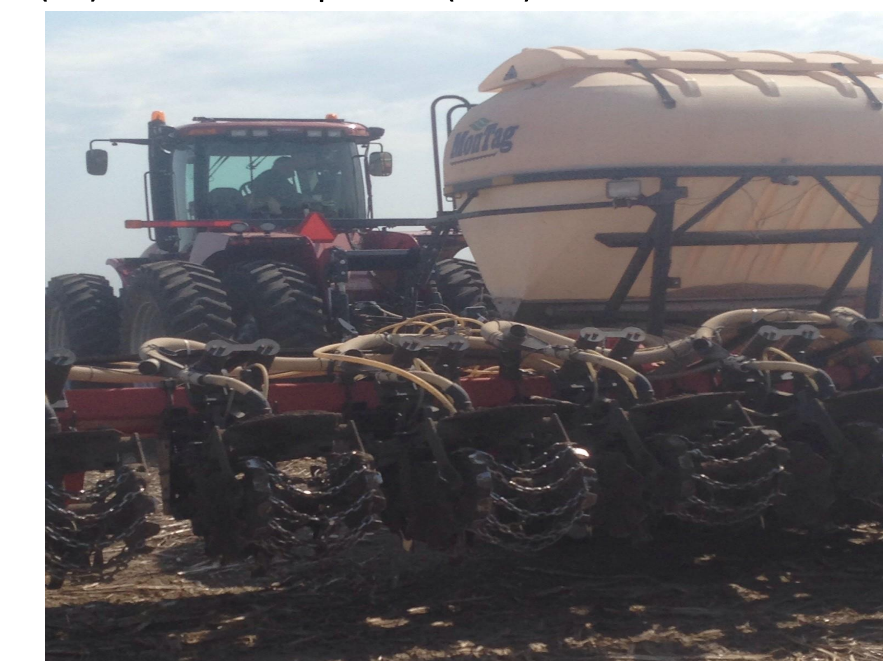
Figure 4. 12 row x 76 cm spaced strip till unit with fertilizer applicator.
