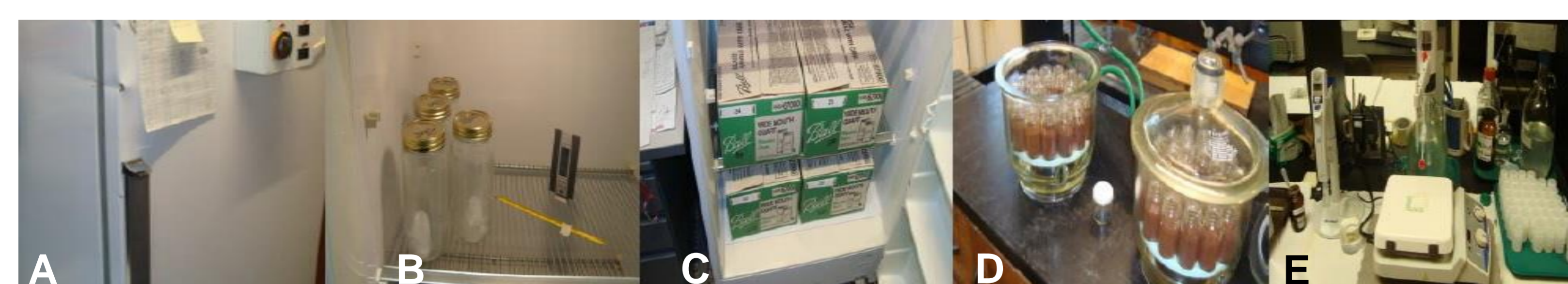
Figure 1. (A) Incubator of the soil samples, (B) Blank sample of each box and thermometers, (C) Boxes with samples inside the incubator, (D) Samples to be fumigated, and (E) Samples ready to be titrated.
