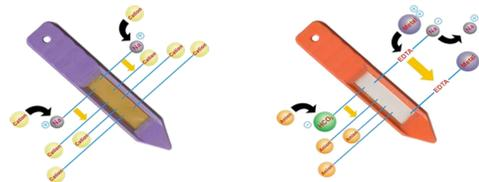
Figure 2. Photos and illustrations of the cation and anion PRS™ probes (Western Ag. Innovations Inc., Saskatoon, SK, Canada) used for *in situ* monitoring of soil nutrient flux.
