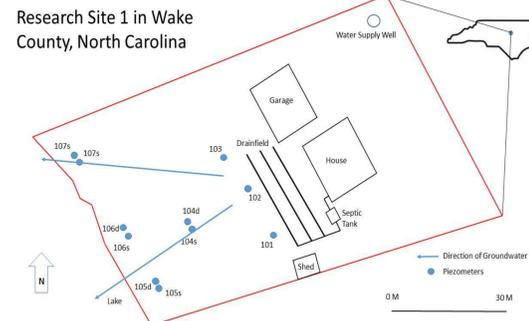
**Figure 2. Piezometers were installed down-gradient from conventional style onsite systems to allow for collection of groundwater samples for nutrient analyses and environmental readings at different distances along a groundwater flow path. Soil samples were collected during the piezometer installations for particle size analyses, CEC, and pH.**
