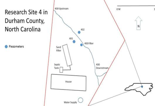
**Figure 3. Piezometers were installed near the sand filter beds of the single pass sand filter systems and away from the beds to determine if effluent from the sand filter was influencing groundwater quality near the filter bed.**
