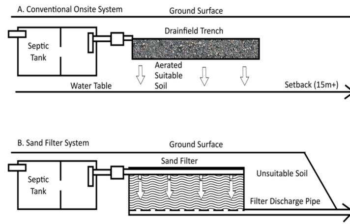
**Figure 1. Diagram of subsurface (A) and surface discharge (B) septic systems. Subsurface systems discharge effluent into the soil beneath trenches, whereas surface discharge systems discharge effluent to a stream/ditch via a filter discharge pipe.**
