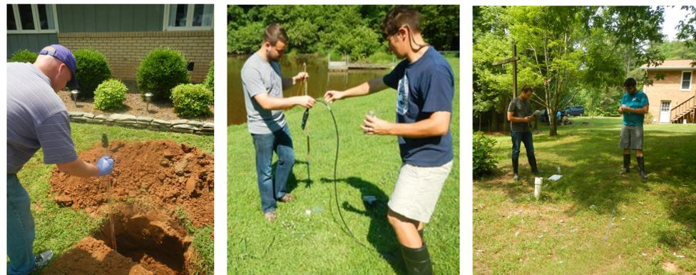
**Figure 4. Septic tanks, piezometers, background wells, sand filter outlet pipes and surface waters adjacent to the onsite systems were sampled 5 times during the study for nutrient analyses and environmental readings. Environmental readings included depth to groundwater, pH, specific conductance, temperature, redox potential, and dissolved oxygen concentrations.**
