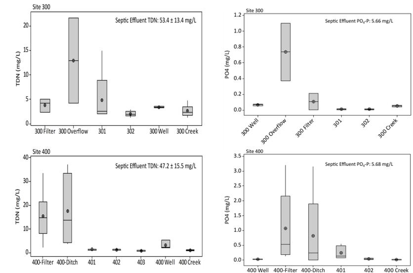
**Figure 6. The concentrations of TDN and PO<sub>4</sub>-P in septic effluent were reduced by an average or 80% and 90% after passing through the sand filters at sites 300 and 400. Mass load reductions of TDN and PO<sub>4</sub>-P were 50 and 83%, respectively for the sand filter.**
