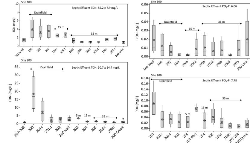
**Figure 5. The concentrations of TDN and PO<sub>4</sub>-P in septic effluent were reduced by an average of 98% and 99% in groundwater 35 m down-gradient from the conventional systems (100 and 200). Mass load reductions of TDN and PO<sub>4</sub>-P averaged 70% and 95%, respectively at these sites.**
