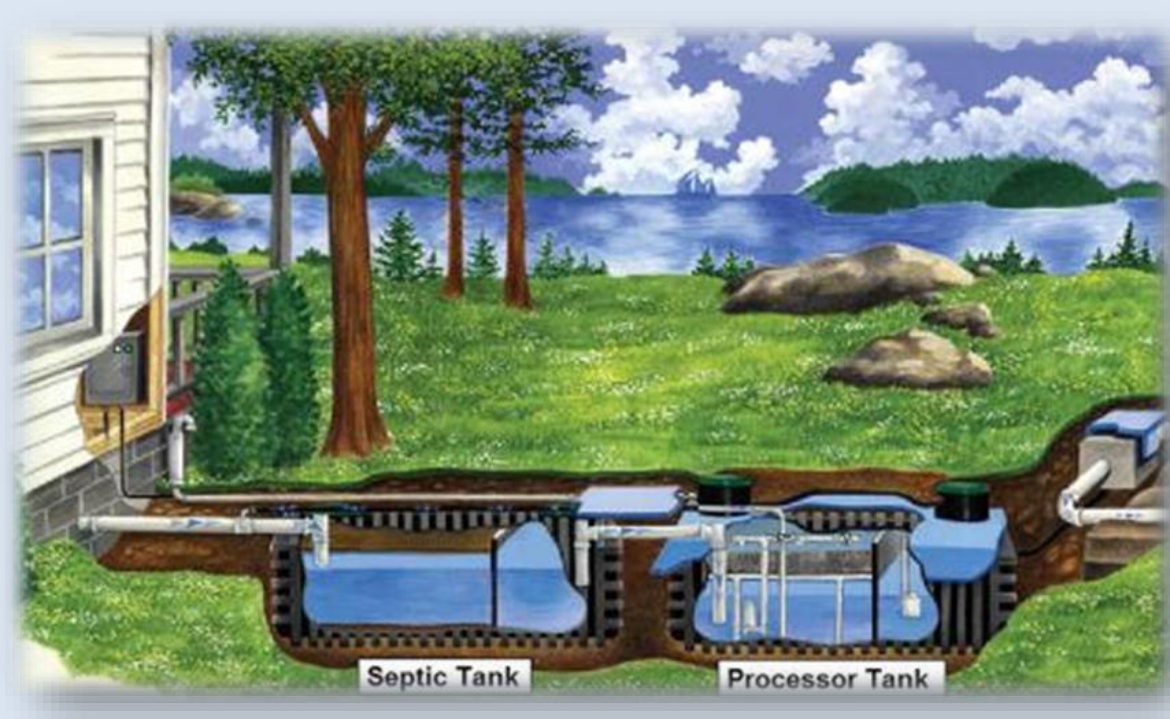
Advanced N-Removal OWTS: 50-75% N Removal
