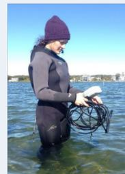
Figure 5. Field measurement of DO, temperature, salinity, and pH were taken using YSI probe
