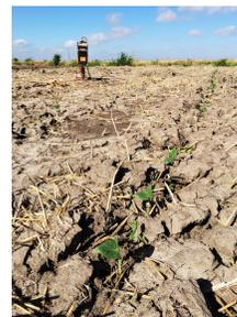
Figure 7. Neutron Moisture Meter takes readings in a conventional till rep with cowpeas as the double crop (Day 215).
