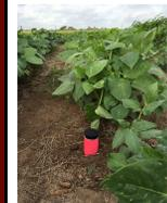
Figure 8. Aluminum access tube (183 cm) for gathering neutron moisture meter data.
