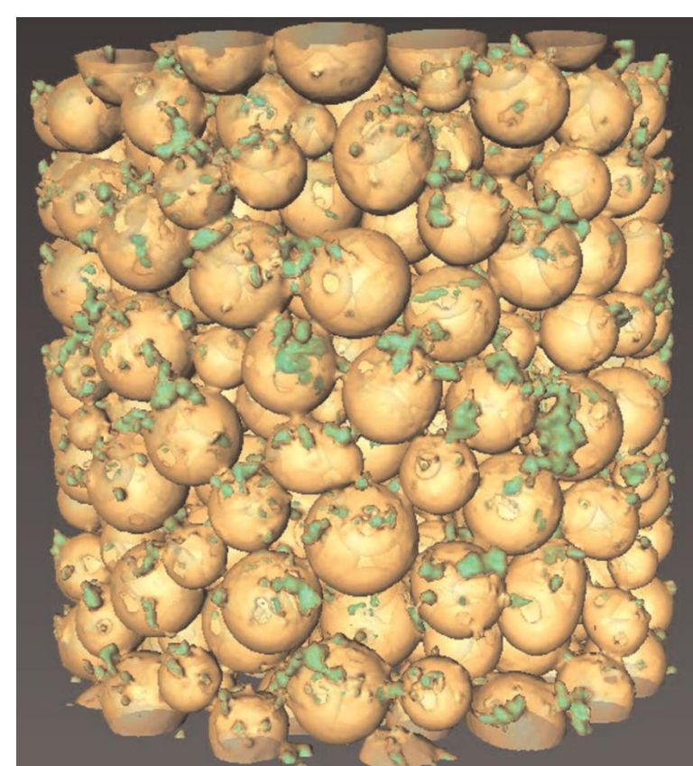
Figure 1: X-ray microtomography imaging of biofilms grown on glass beads (Iltis et al., 2011).
