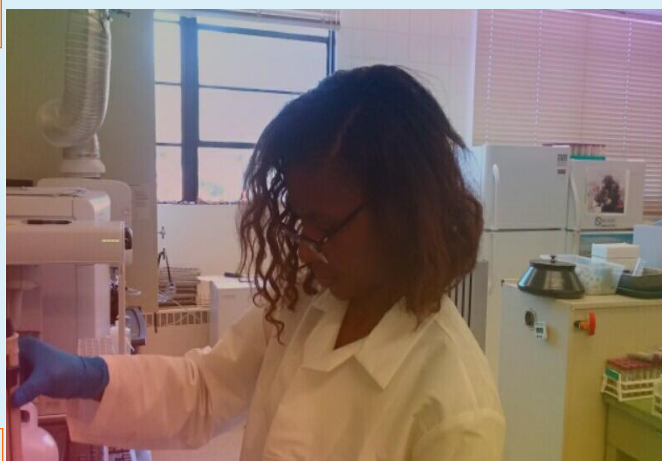
Soil inorganic N (NH 4 and NO 3 ) analysis using KCl extraction
