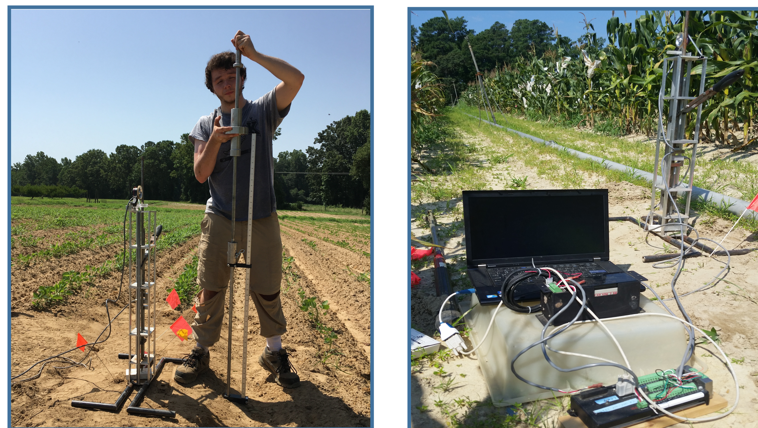
Fig. 1. Photographs of SCP and DCP (left), and the data collection system for the SCP (right).
