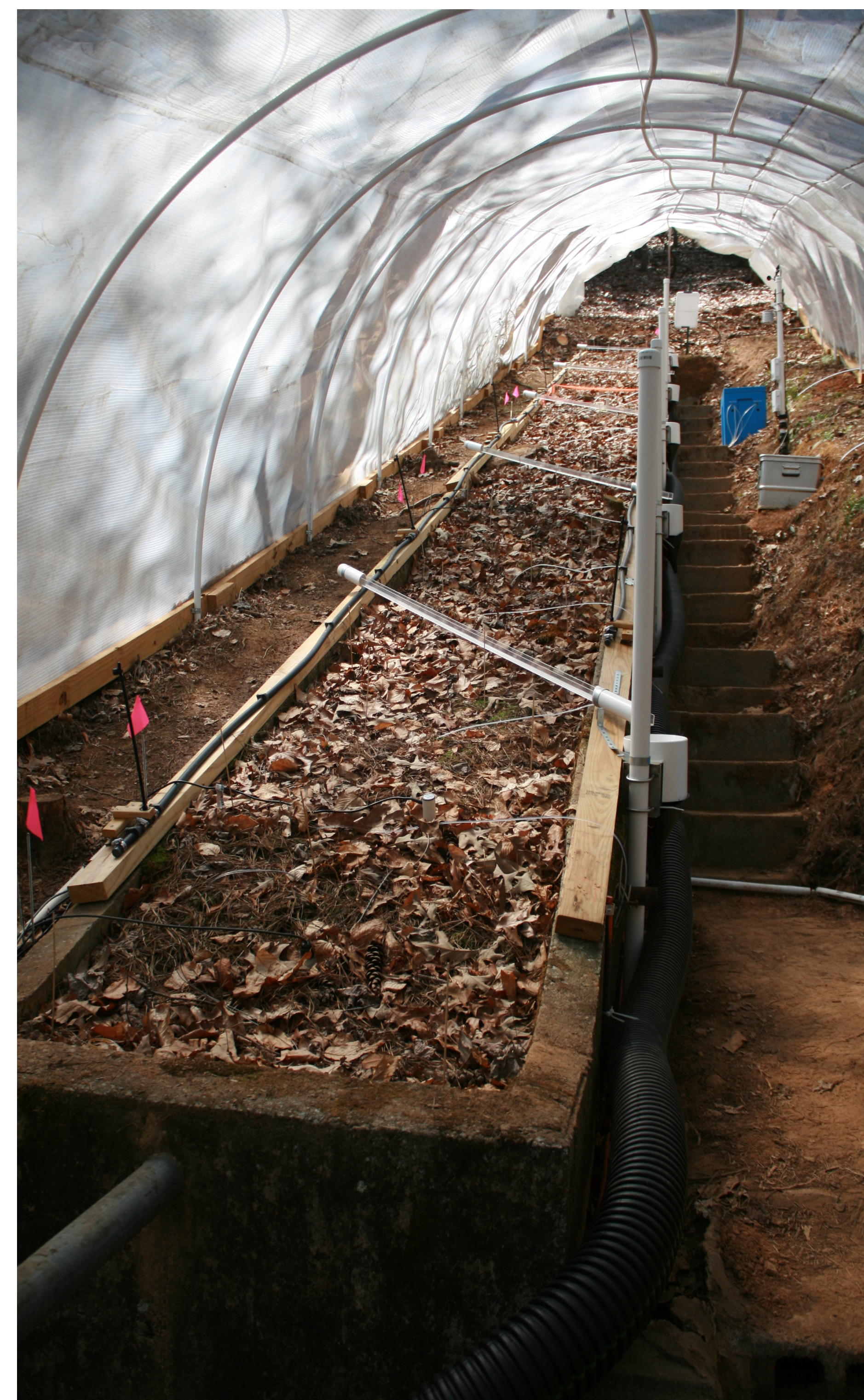
Figure 2 (below). Experimental hillslope soil model at Coweeta Hydrologic Laboratory, USDA Forest Service, Southern Research Station, Otto, NC. The model was originally used to develop the Variable Source Area theory to explain subsurface runoff in hillslope hydrology (Hewlett and Hibbert 1967).
