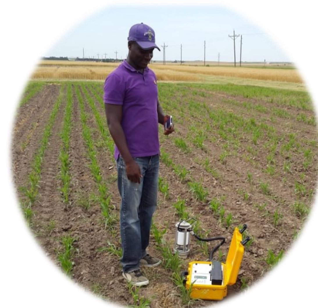
Fig. 1. CO 2 flux measurement in sorghum plot
