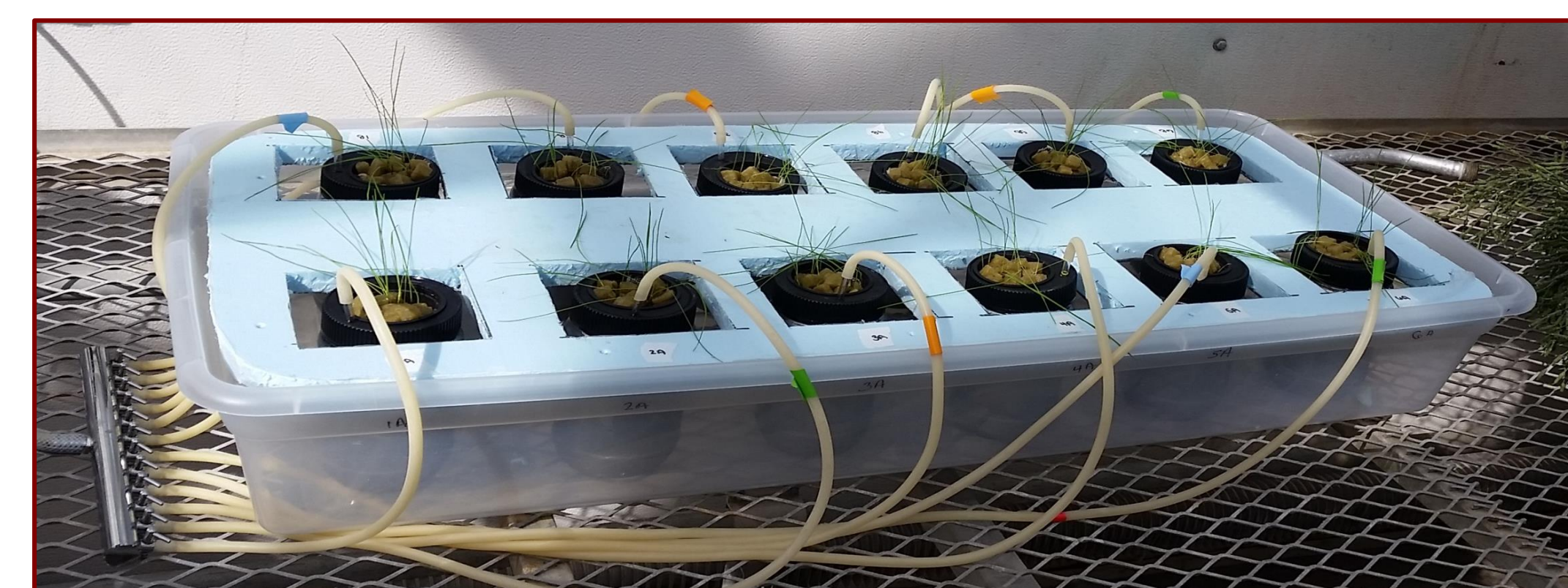
Figure 5. Hydroponic setup with 400 ml containers, aeration tubing, and 15 plants per pot.
