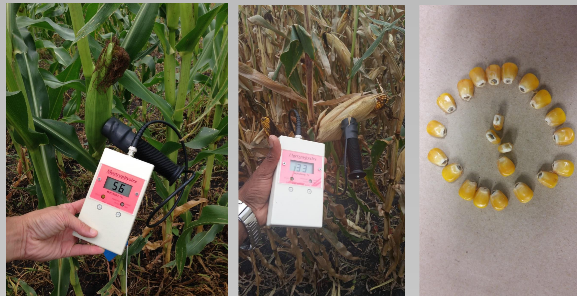
Figure 4. MT 808 electro-physics kernel moisture meter and corn kernels at physiological maturity (black layer)
