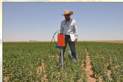
Fig.2. Measuring soil water content with neutron probe.
