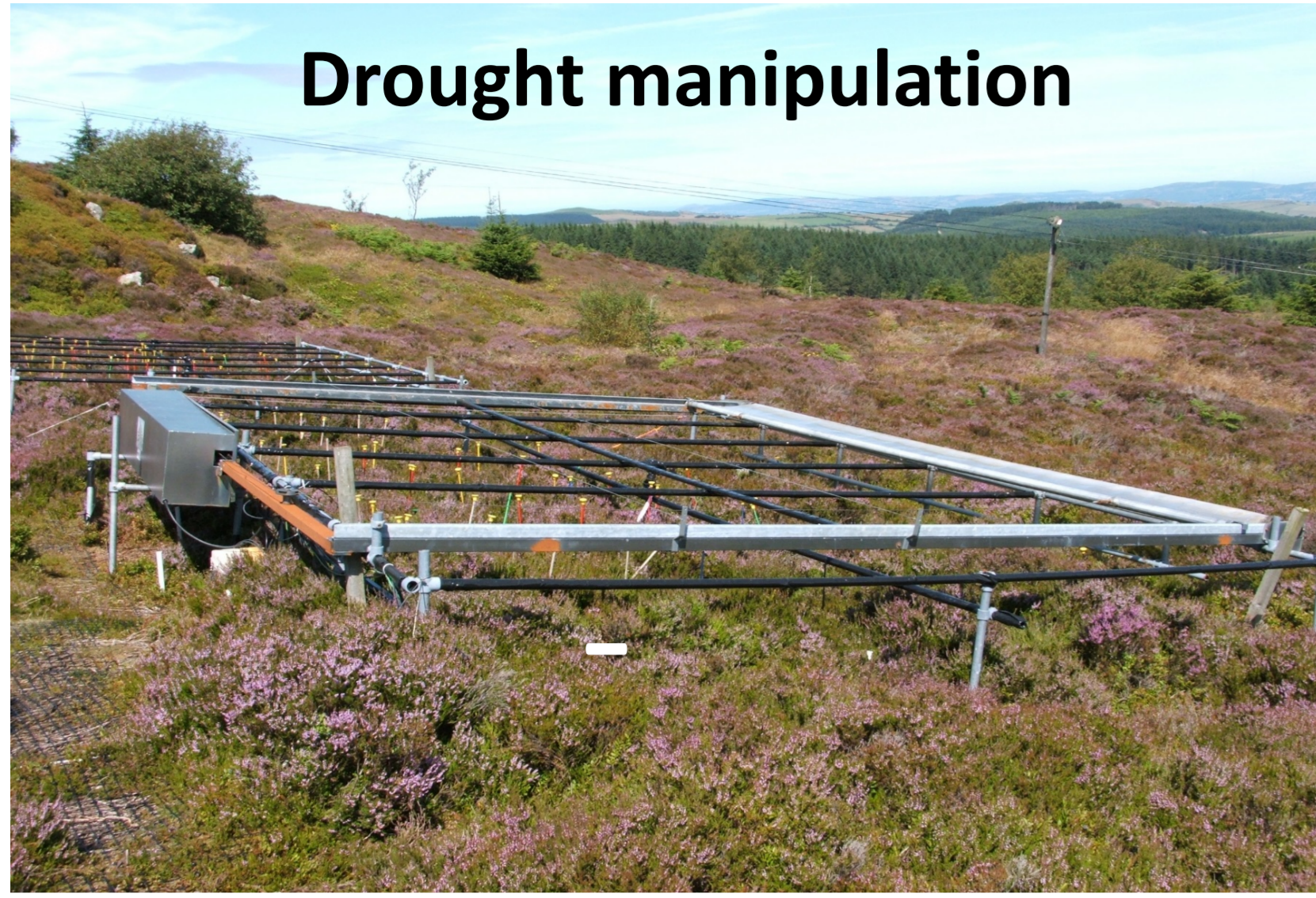
Fig. 1: C. vulgaris dominated experimental field site showing an automated rain exclusion setup.
