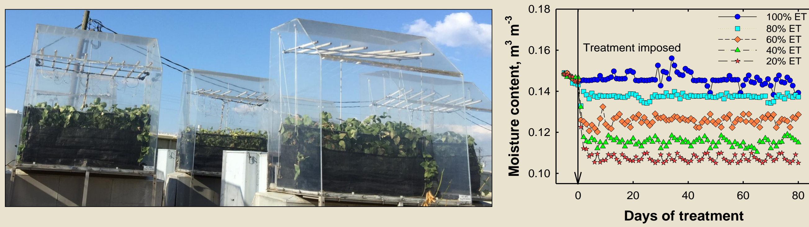
Fig. 1. Pictorial representation of two soybean cultivars grown at 100%, 80%, 60%, 40%, and 20% ET in the Soil-Plant-Atmosphere-Research (SPAR) chambers to study soil moisture stress effects on yield components with the average soil moisture readings.
