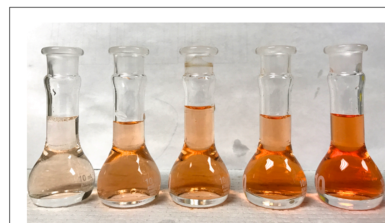
Shades of red in solutions after incubation indicate different concentrations of Fe(II) – phenanthroline complexes
