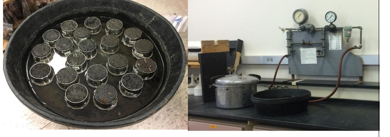
Fig.3. Core samples and ceramic pressure plate for water retention
