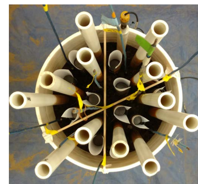
Fig. 2. Completed mesocosm, including reference electrode and Pt electrodes.
