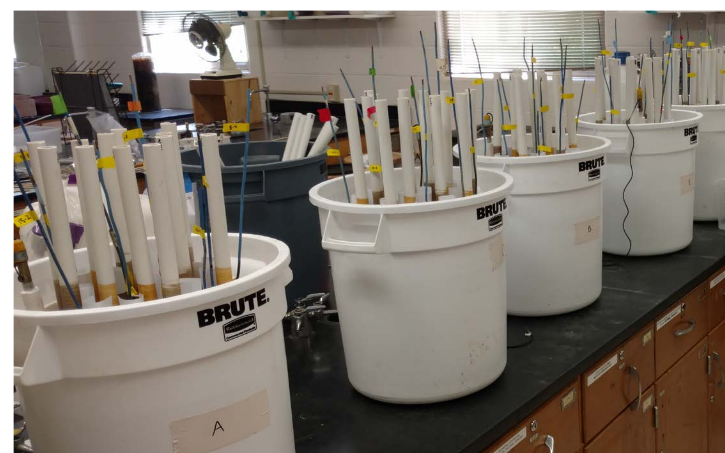
Fig. 3. Mesocosms (19 L buckets, perforated in the bottom) were inserted into larger (38 L) containers for saturation.
