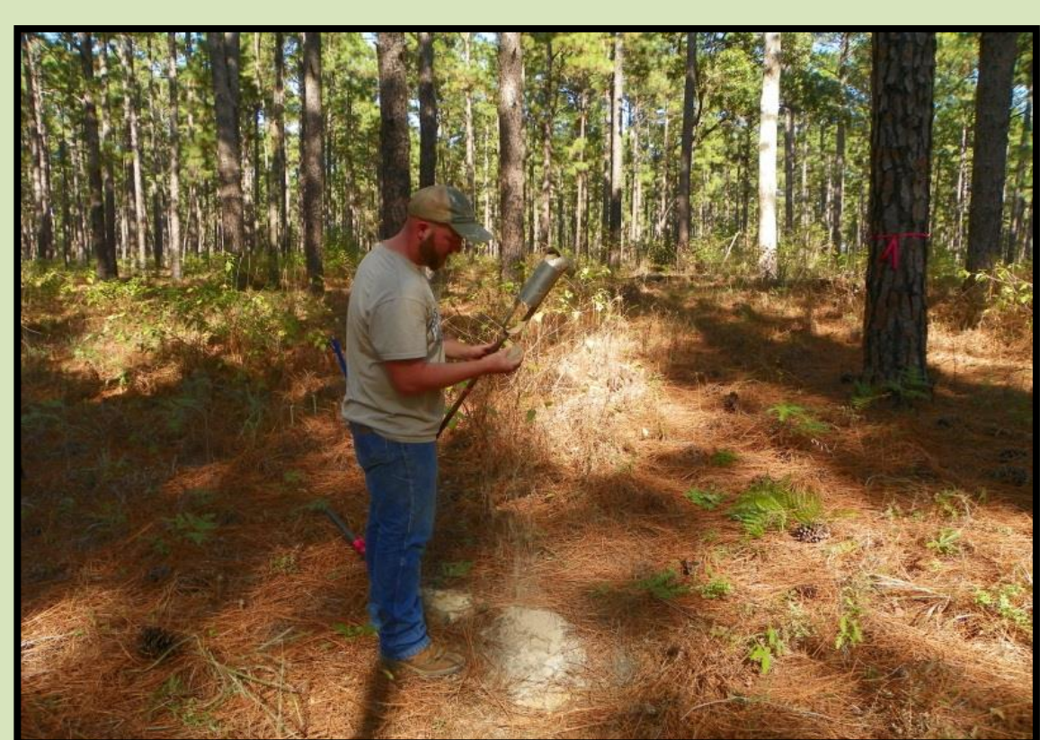
Profile assessment using a three inch bucket auger to verify soil map unit.
