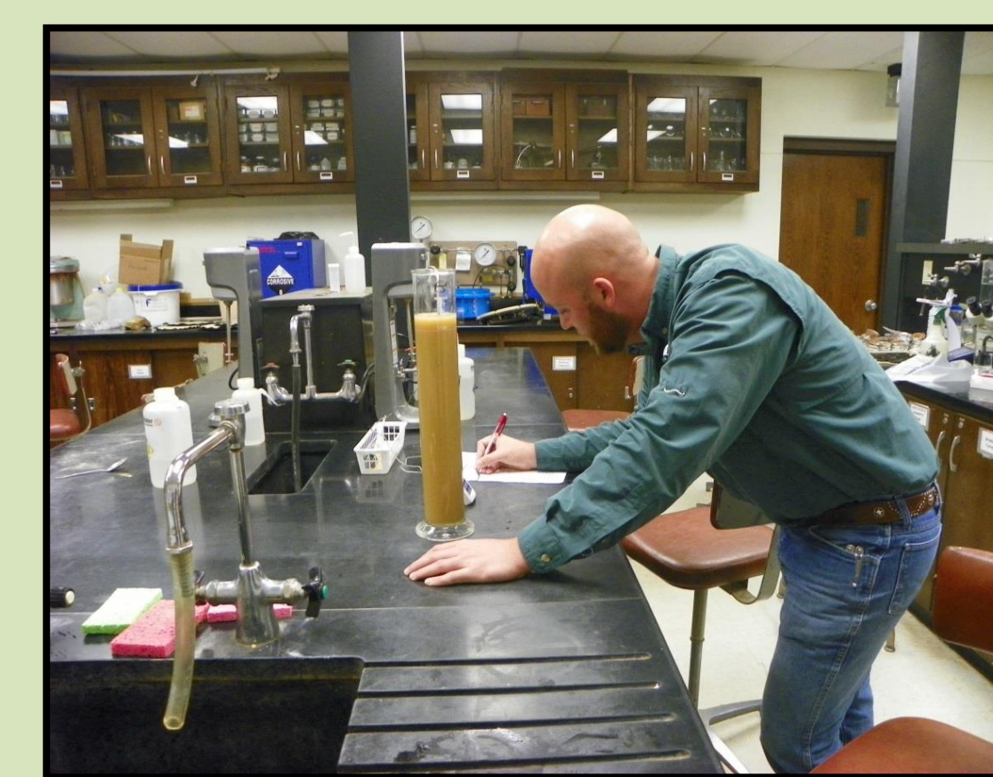
Soil texture determination using the Bouyoucos method.
