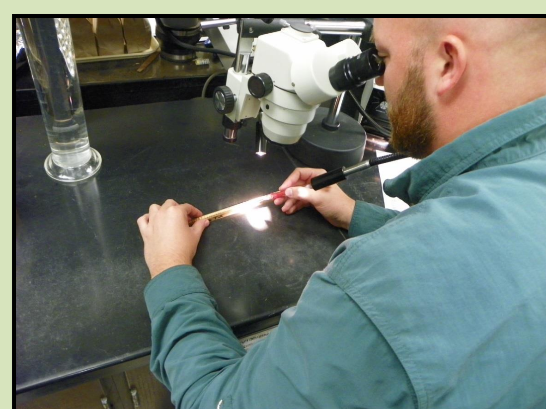
Aging tree cores obtained using an increment borer.
