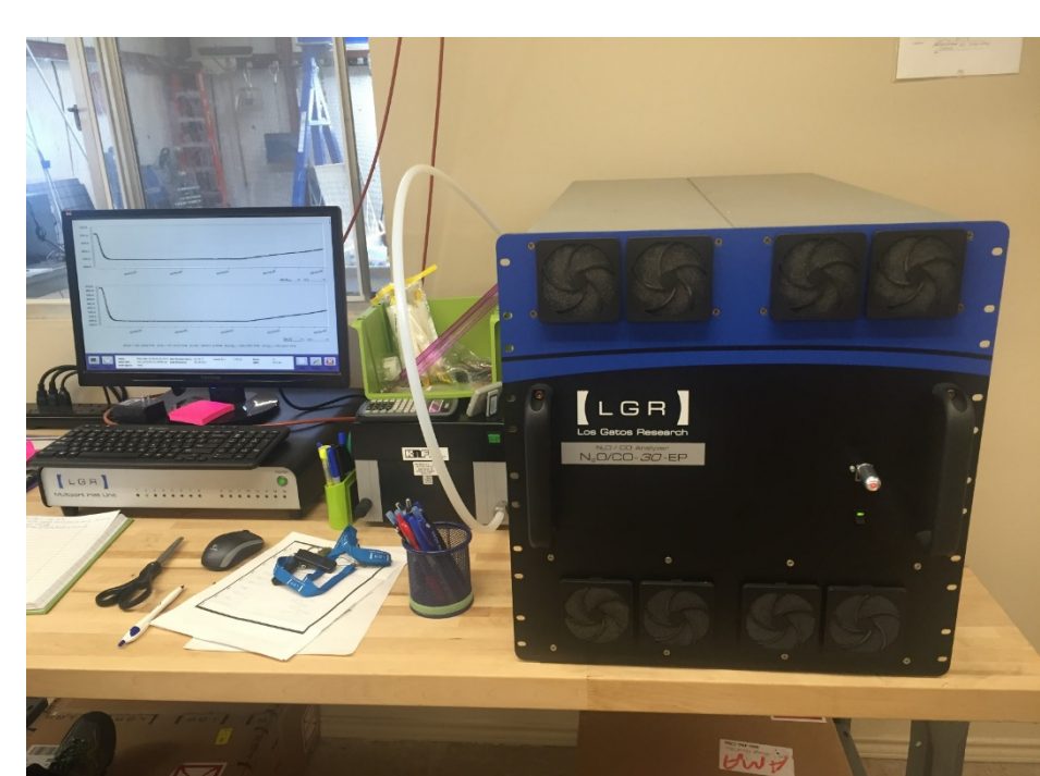
Figure 3. Real-time LGR N 2 O analyzer, multiport inlet unit, vacuum pumps, and standard gases used to quantify N 2 O flux from manure-filled chamber pans.
